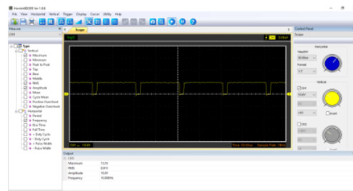
Figure 20. Single energy transfer unit on battery positive side test result
