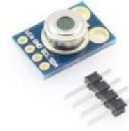
Figure 10. GY-906 Temperature Sensor [27]
