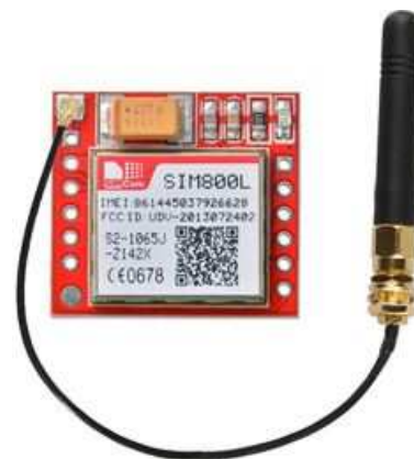
Fig. 4. The module of sim800L GSM [22].
