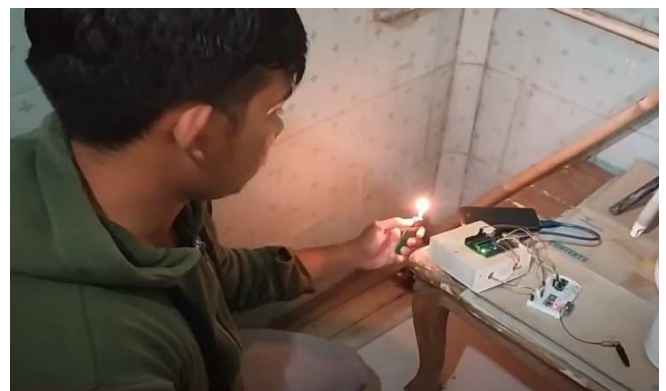
Fig. 11. Experiment using matches to detect a small fire.
