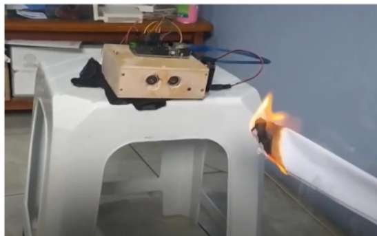
Fig. 12. Experiment using burned paper to detect a fire.
