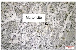
Figure 8. Microstructure at weld metal with WPS
