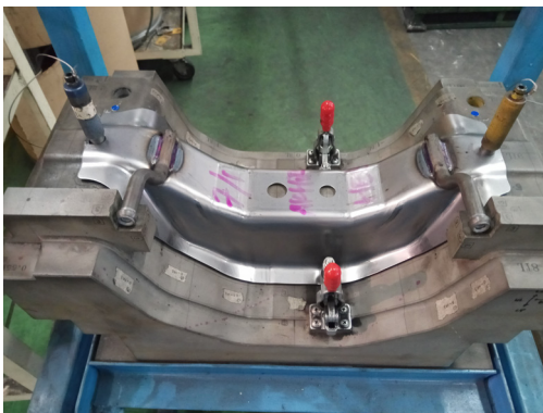
Figure 4. The measurement preparation of welding dimension by jig checking fixture.
