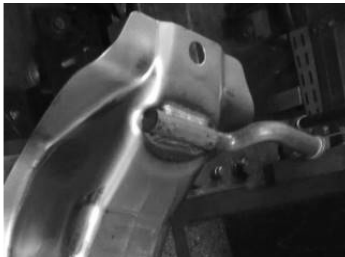
Figure 2. The visual inspection of welding defects on the distortion.
