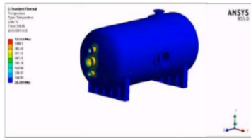
Figure 9. Transient Thermal Load Process of three Cluster Nozzles.
