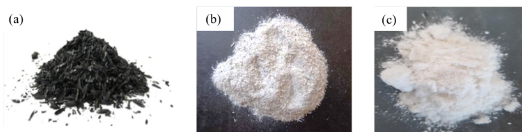
FIGURE 2. Step by step of SiO 2 forming. Burning rice husk charcoal (a) before furnace treatment, (b) after furnace treatment, and (c) dried coarse silica precipitate after sol-gel extraction
