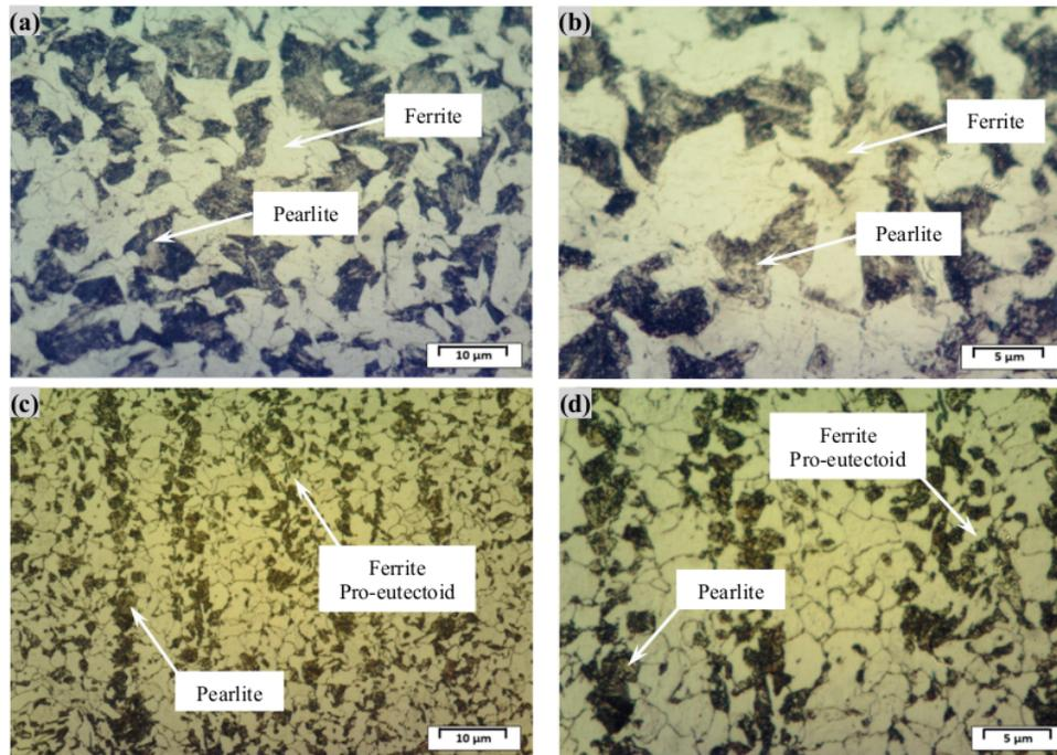
**Figure 3.** Microstructure of SCr420 alloy: (a and b) initial raw before heat treatment at (a) lower and (b) higher magnification, (c and d) after hot-forged at (c) lower and (d) higher magnification.
