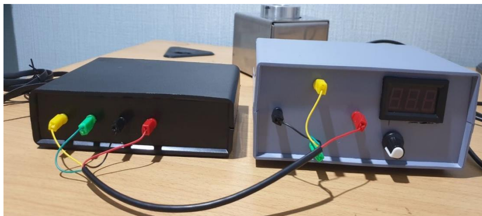
Gambar 2: Pemasangan kabel Wheatstone Bridge
