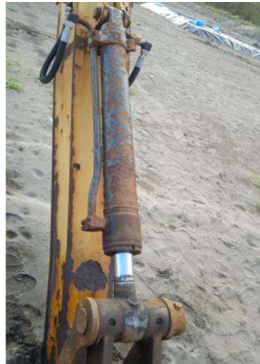
Fig. 3. Corrosion part on the cylinder tube of the housing.
