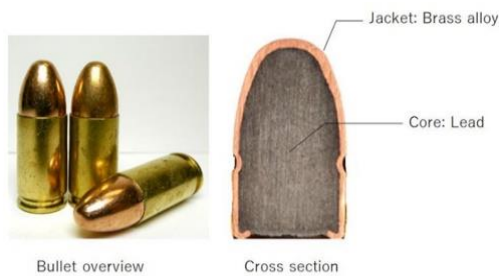
Figure 6. The Pindad MU-1TJ 9mm: A Cross-Sectional View
