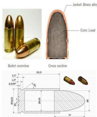
Figure 7. The 9mm bullet: A Cross-Sectional View and Dimensions
