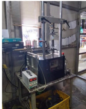
Fig. 9. Experimental setup using damper dynamometer
