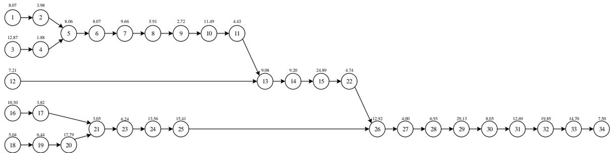
Figure 2. Precedence Diagram of Model A005TG2991ZJ Assembly Process
