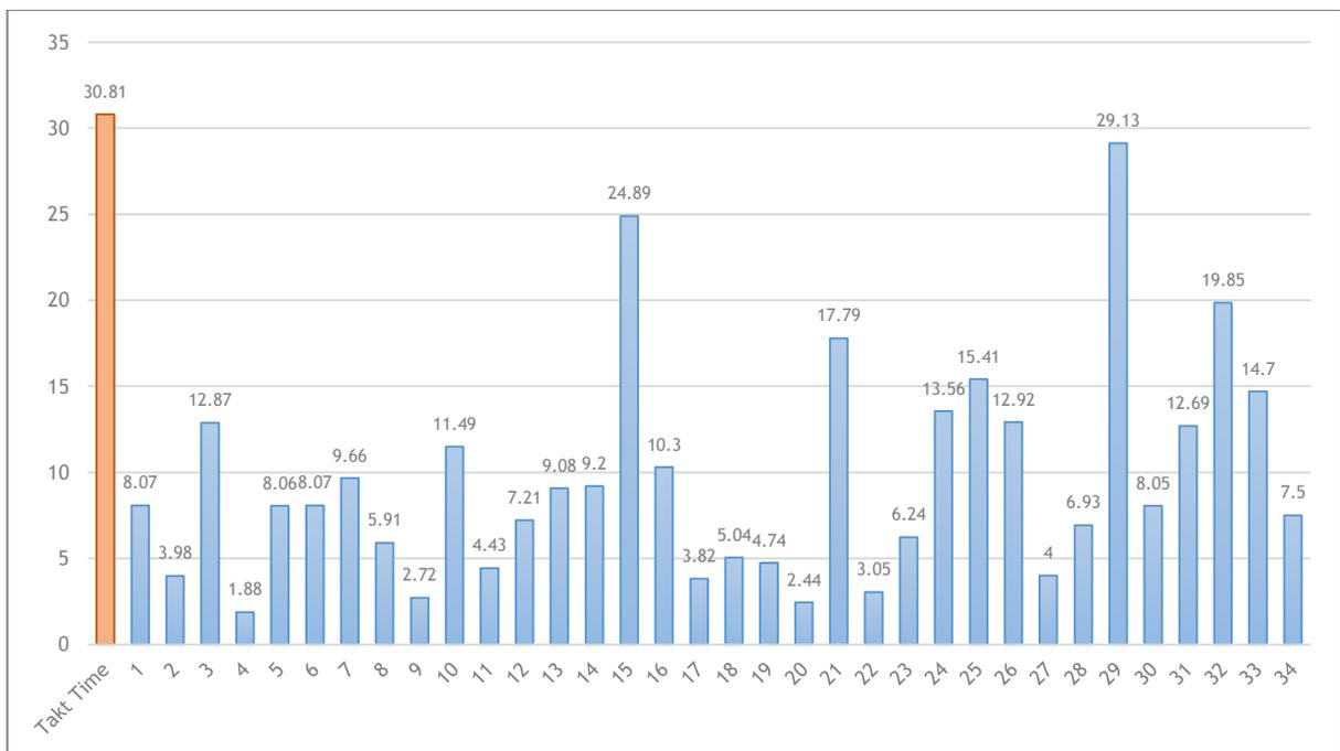
Figure 1. Yamazumi Chart of Assembly Process Model A005TG2991ZJ
