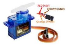
Figure 1. DC Servo Motor [3]
