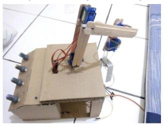
Figure 6. Robotic Arm Design
