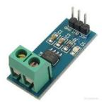
Figure 4. ACS-712 current sensor module
