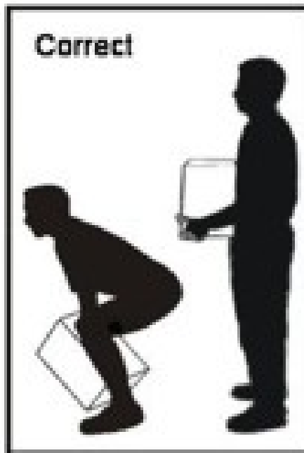
Figure 2.2 Good Practice of Hand Lifting
