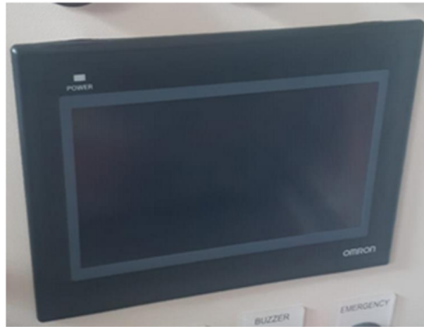
Gambar 6. HMI Omron NB7W-TW01B
