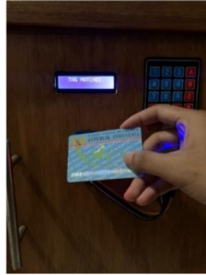
Fig. 14. Point of view scan the RFID card with E-KTP.
