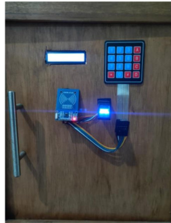
Fig. 9. Full device prototype of 3-level security system (front-view).
