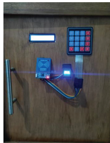
Fig. 5. Full device prototype of 3-level security system (front-view).
