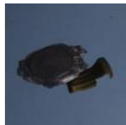
Figure 12. Condition of 9 mm Bullet after Impact
