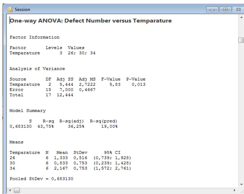
Figure 2. ANOVA Table of Defect Number versus Temperature
