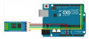
Figure 4. Arduino Uno to HC-05 Bluetooth module
