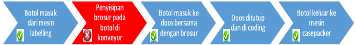
Gambar 4.5 Diagram Alir Proses Mesin Cartonning MA
